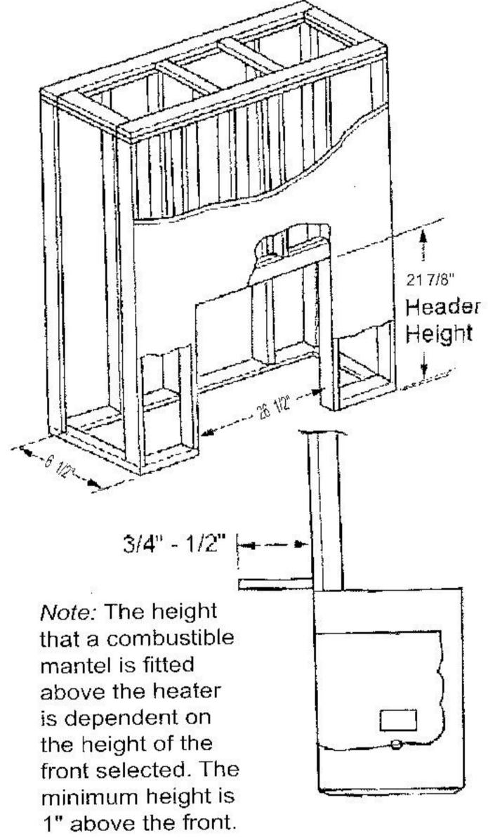
(D) - Framing Heater for New Construction/Renovation
