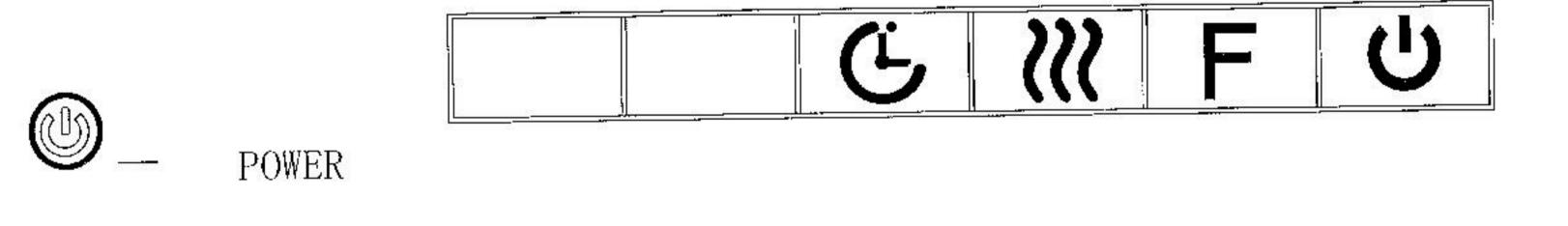
After unit is plugged the power ,Press the power button first time,starting up , touch it second time, the power shut down.
