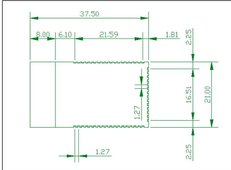
Figure 3 mw302 modules mechanical dimension (Unit: mm)
