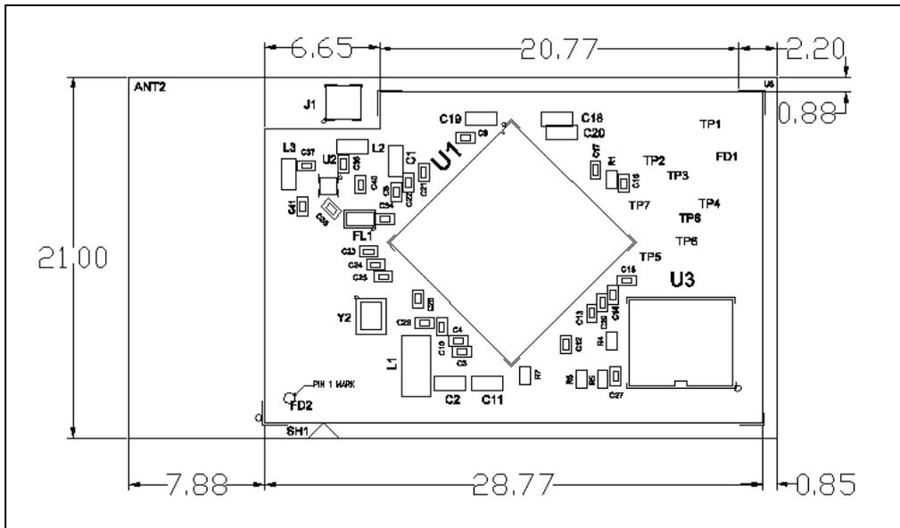
Figure 4 mw302 modules mechanical dimension (Unit: mm)
