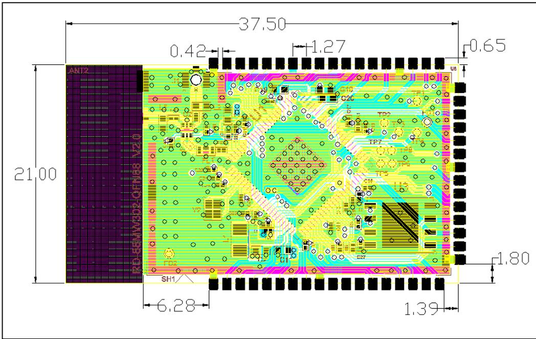
Figure 5 mw302 modules mechanical dimension (Unit: mm)
