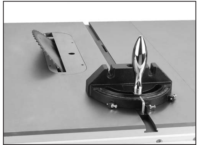
Figure 26. Blade tilted to 45° (guard removed for clarity).
