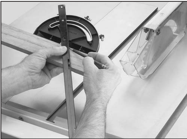
Figure 25. Marking miter line.
