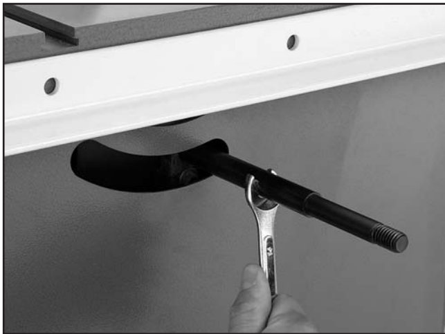
Figure 13. Installing the pivot shaft.
