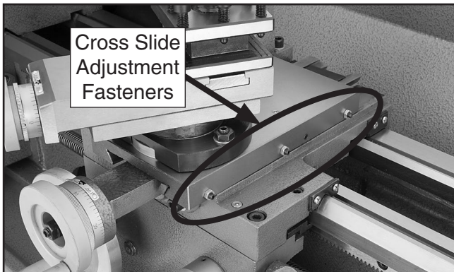
Figure 89. Cross slide gib adjustment hex nuts and set screws.
