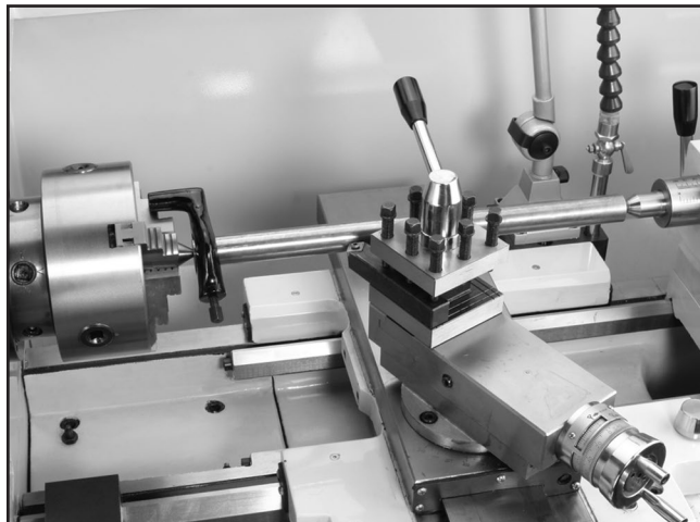
Figure 39. Example photo of stock mounted between the centers.
