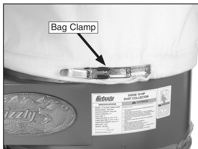
Figure 21. Upper filter bag secured to collector.
