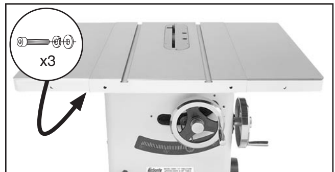
Figure 15. Extension wings installed.
