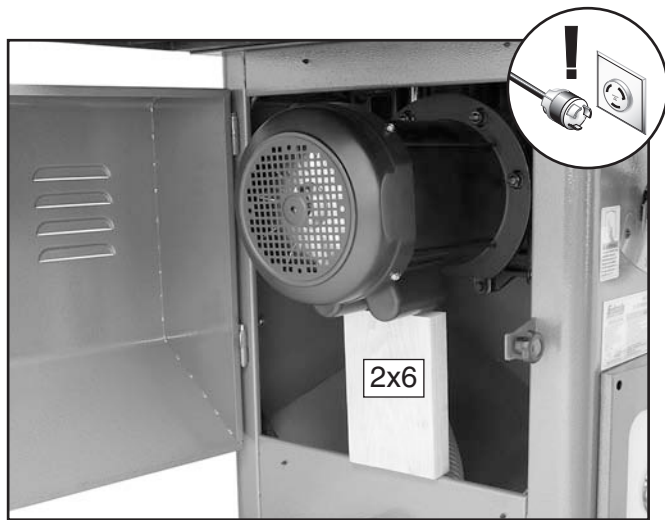
Figure 150. Motor resting on wood block.
