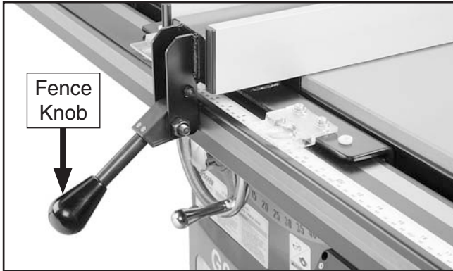
Figure 41. Fence knob installed.
