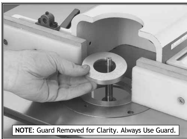
Figure 3. Use the smallest insert the cutter will allow to keep woodchips near the dust collection suction area.
