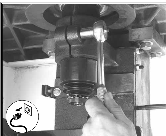
Figure 28. Loosening spindle cartridge bolt.
