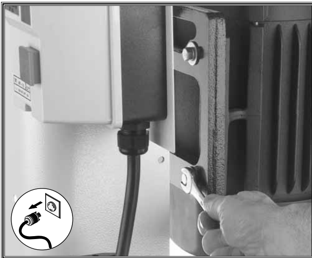
Figure 27. Loosening motor mount bolts.
