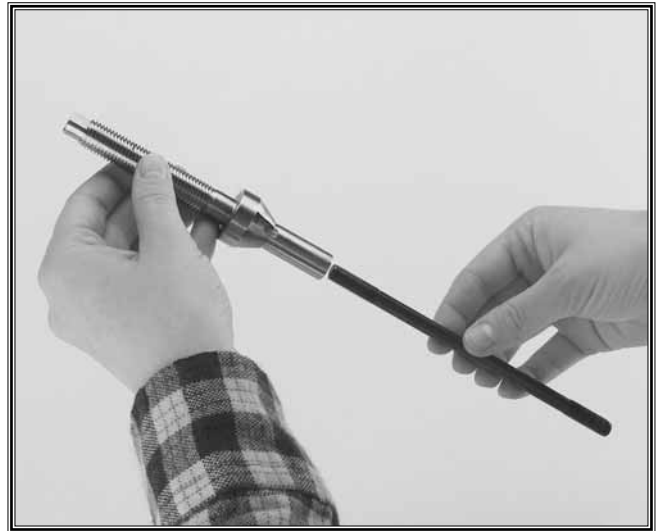
Figure 18. Threading drawbar into spindle.
