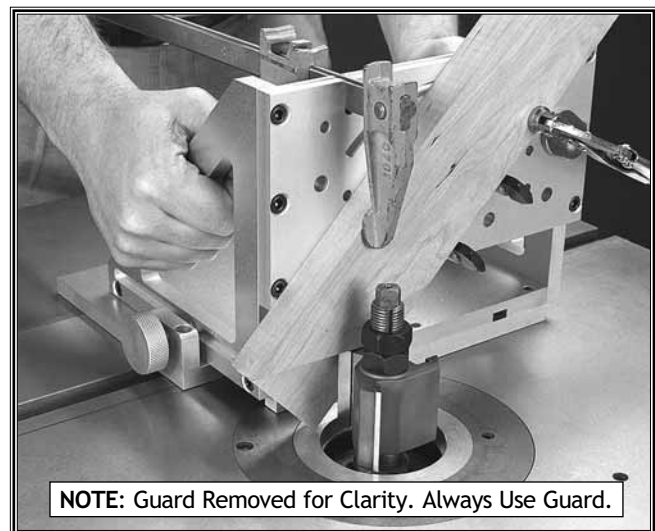
Figure 5. Use a SHOP FOX® Right Angle Jig when making special cuts without a safety guard.
