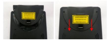
5. Apply the back cover screws to fasten the Expansion Module.
