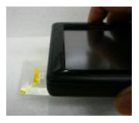
Position handheld parallel to the tag. Keep scanning distance within 3cm.
