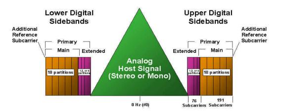
Figure 4.10: Hybrid spectrum allotment of FM HD Radio system
