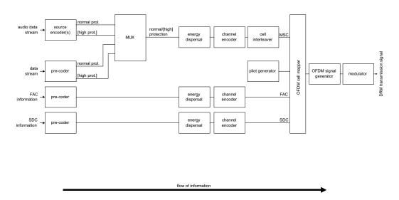
Figure 4.1 depicts the general flow of different classes of information (audio, data, etc.) after their origination in a studio or control centre (that would be depicted to the left of the figure) to a DRM transmitter exciter/modulator on the right. Although a receiver diagram is not included in the figure, it would represent the inverse of this diagram.
