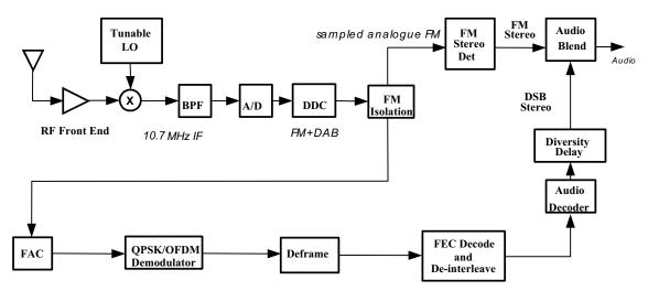
Figure 4.15: FM hybrid IBOC receiver functional block
