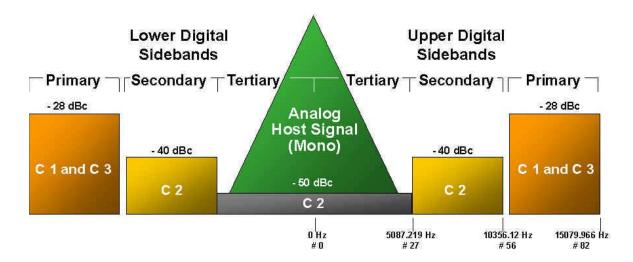
Figure 4.12: Hybrid AM HD Radio system spectrum allotment
