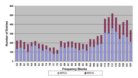
Figure 4.20: Estimation of the channel usage in Band III for T-DAB (RPC4: suitable for mobile reception; RPC5: suitable for portable indoor reception)
