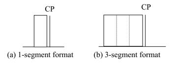
Figure 4.8: CP carrier in connected transmission
