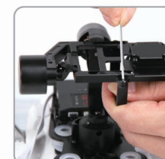
5.2 Unscrew 2 M2x4 screw, Loosen the camera fixed frame.
