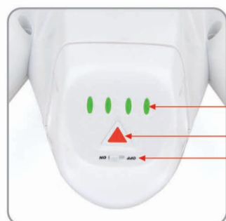
2.4 Turn the power switch to "ON" position, and press on the power button about 3-5 second till the green LED light solid. The undercarriage(skid landing) will unfold automatically.
