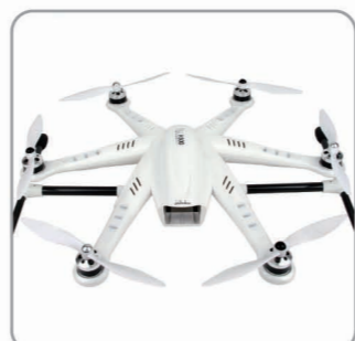
1.3 Propellers Installation finished.
