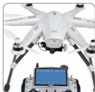
3.6 Put aircraft to the horizontal position, the Red LED and Green LED light out which means calibration finished. Please reconnect the aircraft power after calibration.
