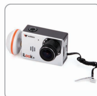
5.1 Screw the camera mushroom antenna into Camera.
