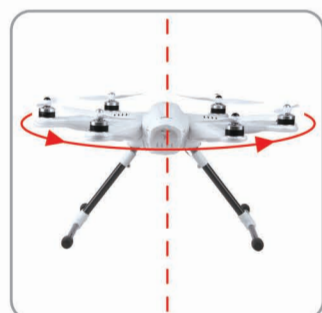
3.4 Horizon level 360° rotation (Rotate the aircraft, from 0° to 90°, 180°, 270°, 360°, all need to pause for 1 second.)
