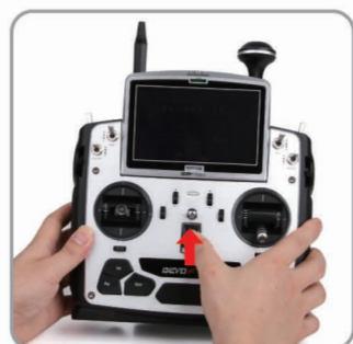
2.3 Turn all the Switch of transmitter to "0" Position, push the throttle stick to the lowest position, Turn on the transmitter power.
