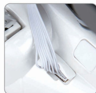
4.5 Insert 9 pin of the Gimbal date wire into the Gimbal connection port at the bottom of the aircraft.
