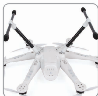
2.5 Put aircraft to the horizontal position, the Red LED and Green LED flash till light out which means code binding successful.
