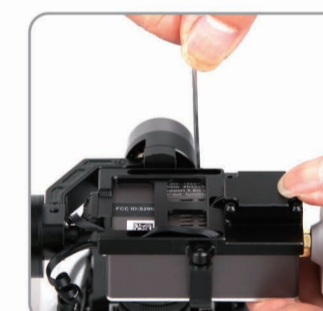
5.3 Install the camera into gimbal, Fix it with camera fixed frame (ensure the gap close to the lens), then screw the M2x4 screw to the camera fixed frame again.
