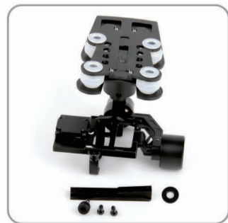
4.1 Prepare the G-3D gimbal, Gimbal fixed block, gasket, screw, spring.
