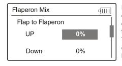
Press DN to display Flap to Flaperon setting interface, and press UP or DN to move the Navigation mark to choose "UP or Down" setting options. Press R or L to change the Flaperon Mix value when moving the Flaperon stick. The bigger the Value is, the bigger Mix will be . The adjustable Mix is ranged from -125% to +125%. It is possible to change the Flaperon Mix direction by changing the plus or minus sign before the value.
