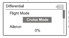
Press ENT to enter Main Menu; Press UP or DN to move the navigation mark to Function Menu, and press ENT to enter Function Menu. Press UP or DN to choose Differential and Press ENT to enter Differential interface. Picture as left:
