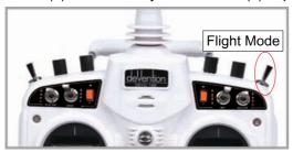
The settlings for Cruise Mode, Speed Mode, Thermal Mode, Launch Mode and Land Mode 5 are available.
