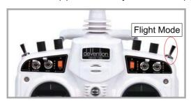
The setttings for Normal Mode, Stunt 1, Stunt 2, Stunt 3, Stunt 4 and Throttle Hold are available. But for Stunt 3 and Stunt 4, Flight Mode Extra Switch at Device Select in Mode Menu should be activated(Refer to "2.9 Device Select"), and Throttle Hold in Function Menu should be set as Active(Refer to "3.5 Throttle Hold" below).
