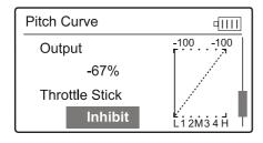
Throttle Stick setting: Press UP or DN to select Throttle Stick seting, Press R or L to increase or decrease, respectively. The adjustable range is from 0.0% to 100.0%. Choose Inhibit and the throttle stick will not be set as a switch.
