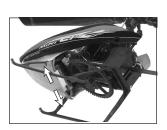
Step 1: disconnect the power cable of helicopter.
