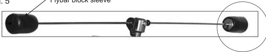
Fig. 5 Flybar block sleeve
