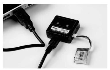
To charge the flight battery, first plug the Mini-USB charge cord into the 500mA DC USB Dual Port Charger. Then plug the standard USB end into your computer or other suitable 5V USB outlet. The LED will start GREEN and when you plug the flight battery into the charger the LED change to RED. When the charge is complete the LED returns to GREEN.
