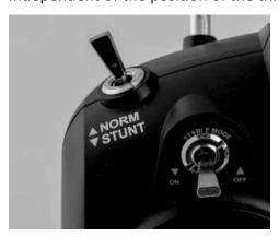
tle stick movement above mid point engages positive pitch on the main rotor, any stick movement below mid stick produces negative pitch on the main rotor allowing you to fly inverted. For 3D flight, Idle Up should be engaged once you have taken off in Normal mode and established a stable hover. Use caution, engaging Idle Up brings the main rotor to full power.
