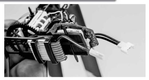
Slide the charged LiPo battery into battery holder with the wires to the front of the helicopter. With battery in place and the transmtter turned on, plug battery into control board making sure that you have the polarity correct (red wire to red wire).
