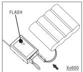
2. With the system hooked up as shown, insert the bind plug in the charge plug receptacle. Turn on the power of the receiver  $(4.8 \sim 5.6 \text{v})$ , and now LED(xy600) should be flashing indicating that the receiver is ready to bind.
