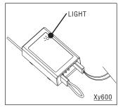
3. LED(Xy600) should be go solid, indicating the system has connected.
