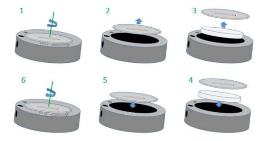
Note: only the same CR2016 3V lithium batteries should be used for replacement, to avoid installation failure or damage to the RM1.
