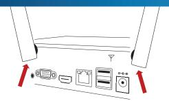
1 Connect the two included antennas to your wireless NVR. This will ensure you achieve the maximum wireless range for transmission from your wireless cameras.
