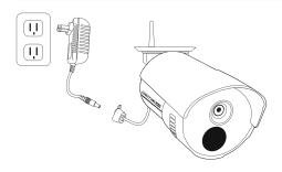
it Each camera comes equipped with its' own camera power adapter. Connect the female power cable coming from the camera to the male power end of the camera power adapter. Next, plug the camera power adapter into a wall outlet.
