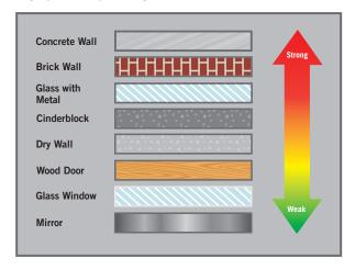
**NOTE:** If your setup requires the signal to be transmitted through an obstacle that severely weakens it, you can use the 9 ft. Wi-Fi Extender Antenna included with your system. The Extender Antenna can be used to bypass the obstacle weakening the signal. Simply replace the white Camera Antenna with the Extender Antenna and then mount the Extender Antenna on the opposing side of the obstacle.
