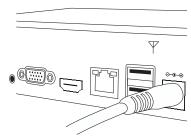
**7** Connect the Wireless NVR power adapter to the Power Input on the rear of the Wireless NVR.
