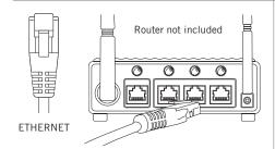
5 Plug the other end of the Ethernet cable into a port on the back of your router.
