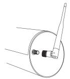
**9** Connect the included camera antenna to the antenna mount on the camera.
