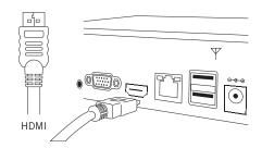
2 Plug one end of the included HDMI cable into the HDMI port on the back of the Wireless NVR.
