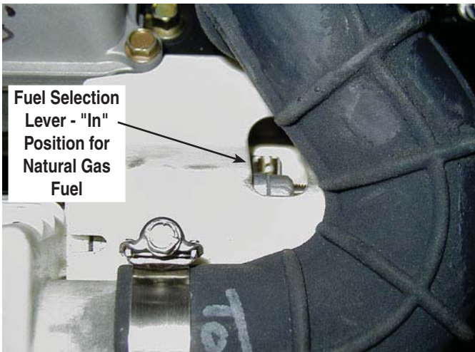
Figure 1.6 - 10kW, GT-530 (Inlet Hose Slid Back)
