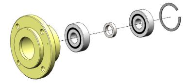
7. The side plate side bearing assembly (clear zinc plated) is shown below.
