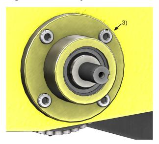
4. At this point remove the bearing housing from the sideplate using the 13mm socket or wrench
