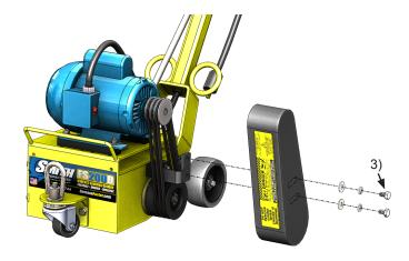
4. Loosen (do not remove) the four nylock nuts locking down the engine until the engine slides freely using the 1/2" socket for the belt side nuts and the 9/16" socket for the side plate side nuts
