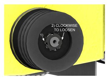
3. Once the pulley is removed, the bearing assembly on that side can be removed using the 6mm hex key.
