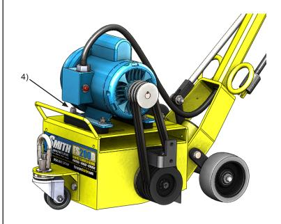
5. Slide the engine back enough to remove and replace the belts as necessary.
