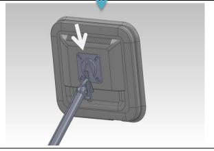
The touchscreen monitor has a Monitor Mount Retainer bracket installed on its rear side. Slide the holding clamp of the Monitor Arm into the matching slot on the bracket to install the Monitor. It will snap into place when installed correctly.
