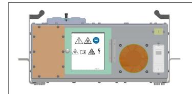
Close the Bulb Access Door and replace screws. Save packaging; lamp assemblies require replacement after 1000 hours of use. Return used lamp assemblies to Guided Therapeutics, Inc. for recycling and disposal.
