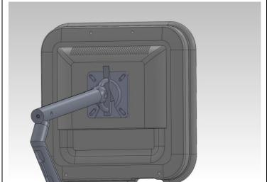
To remove the Monitor, press the monitor clamp and slide the monitor upwards.
