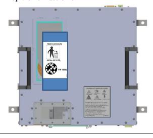
Remove any protective covering from the top of the base unit.
