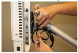
Thread the cables through the cable holders on the monitor arm. Connect the cables to the inputs marked on the monitor.
