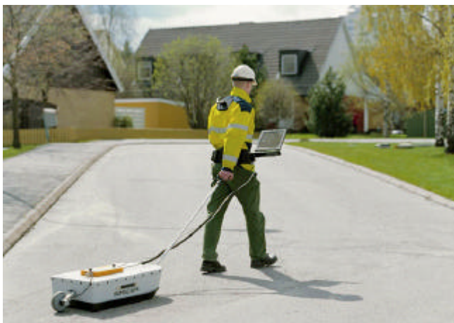
Figure 5.2. RAMAC/GPR Cart with X3M and 250MHz antenna.
