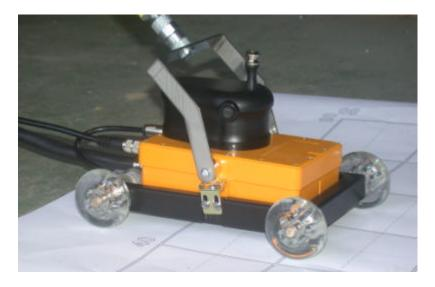
The RAMAC 1.2 GHz antenna communicates with the control unit CUII through a 3 m long data cable, giving you an easily and freely movable antenna.
