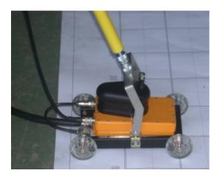
When the 1.2 GHz system is used together with the RAMAC XV11 Monitor, you have access o the fully integrated data collection, 2.5D analysis tool and Migration Wizard.
