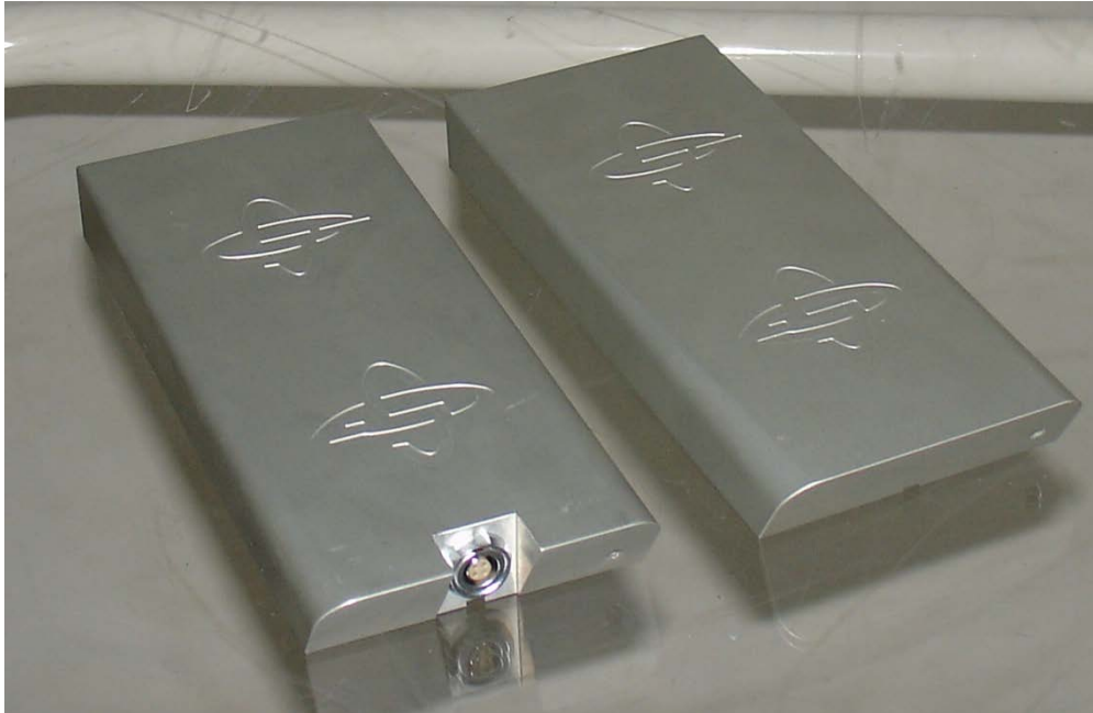
Figure 2, dummy-battery and normal LI-Ion battery.
