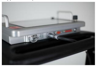
Press and release the button the GPR-transducer, shortly, do keep it pressed. This will start up the unit; the LED's on the panel will start to blink as well as the LED inside the button, see figure below.
