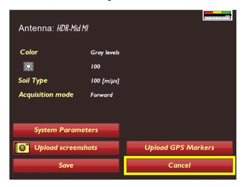
Activating the green text-fields, but turning the push-turn button, and then depressing it gives the user means for changing the settings. Below the different options are described.
