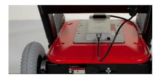
Connect the Monitor to the transducer with the cable supplied, see picture below.
