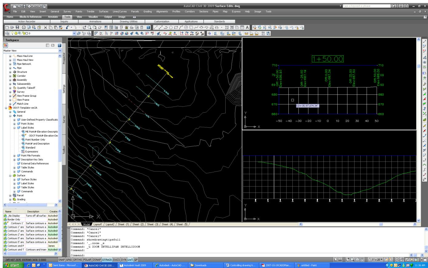
Notice I place my cursor in the section view. A temporary line is drawn in the profile and alignment views at that specific station.
