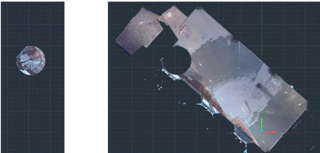
After specifying an appropriate cropping boundary from one view (such as plan), change to another view (such as elevation) to intuitively specify the cropping boundary for the height. You can continue to change views and create cropping boundaries to focus on just the area of the point cloud that you need.
