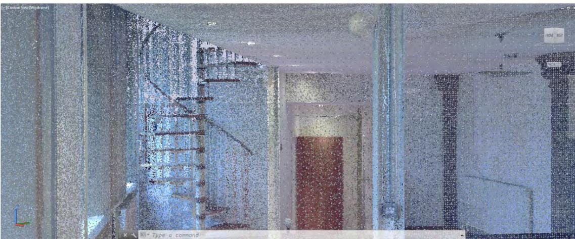
The Autoupdate tool was removed and the previous Density and Realtime Density sliders were replaced by a single Level of Detail slider. The Level of Detail sets the density for all point clouds in the drawing and is relative to the maximum points as specified on the 3D Modeling tab of the Options dialog box. The maximum points displayed on-screen has increased in AutoCAD 2015 from 10 million to 25 million.
