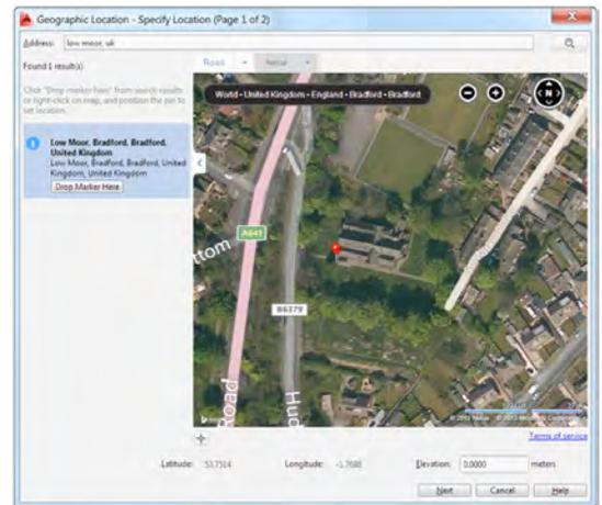
When you're satisfied with the location, the Next button leads you to the second page where you specify the coordinate system. Based on the marker location, AutoCAD 2015 lists only relevant coordinate systems. You can use the search field to further filter the relevant coordinate systems selecting the most appropriate one.
