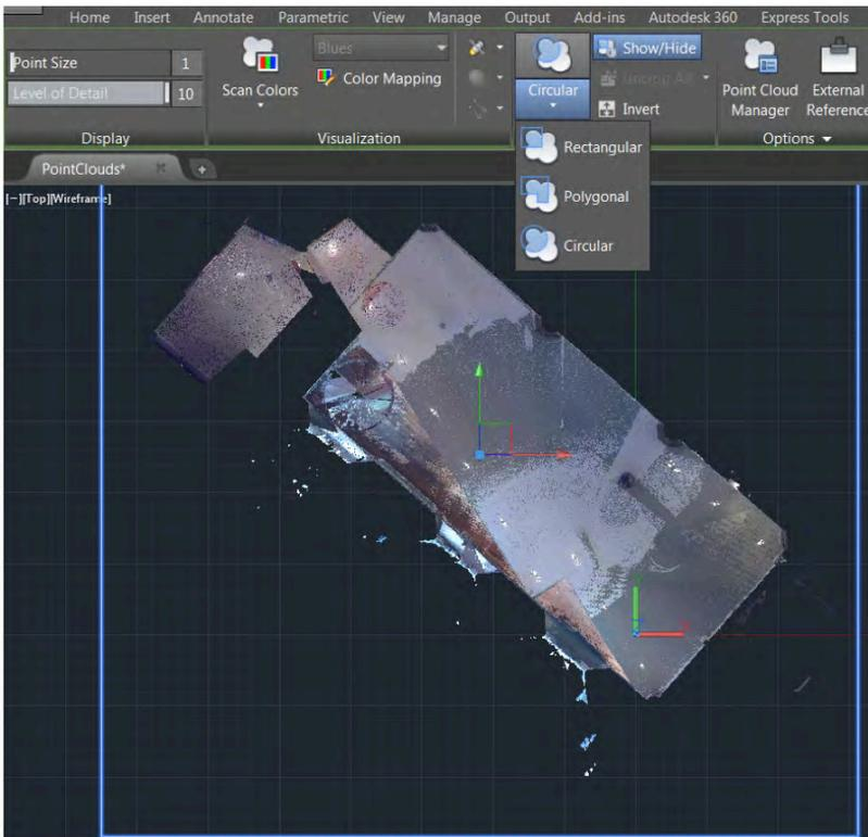
The Invert tool enables you to easily invert the specified boundary to reverse displaying points inside or outside the boundary.
