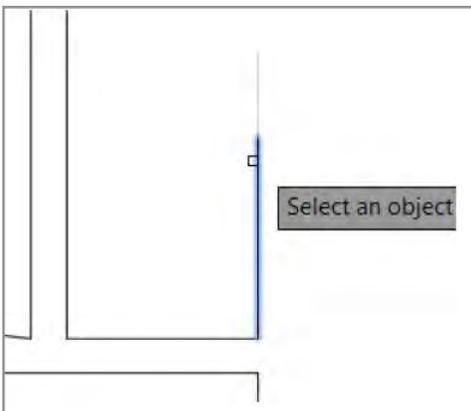
The Break tool displays the results of the Break operation prior to specifying the second break point.
