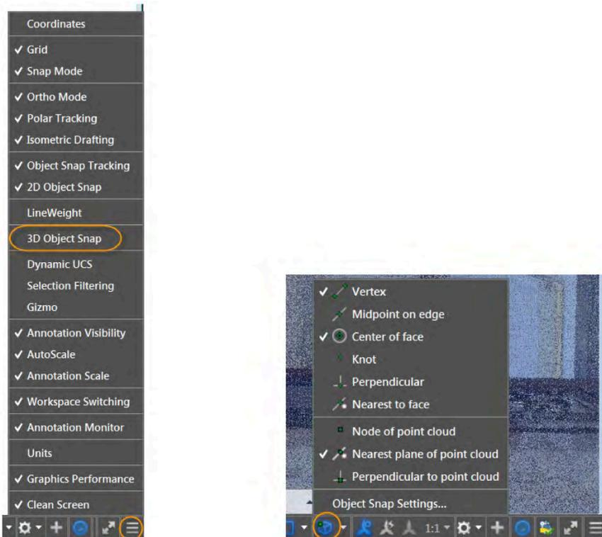
You can snap to points on the point cloud with the Node point cloud object snap. If the point cloud has segmentation data, you can snap to the nearest point on planar segments or perpendicular to planar segments.
