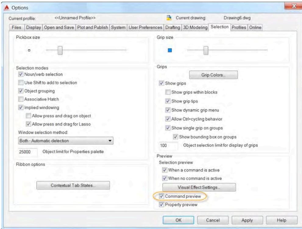
The Trim and Extend tools are enhanced in AutoCAD 2015 to provide a preview of the results before you commit to the selection. After you select the cutting or boundary edges, you simply pass the cursor over the object you want to trim or extend. A preview of the resulting object is displayed. When trimming, the segment to be removed is dimly displayed and a cursor badge indicates that it will be deleted.
