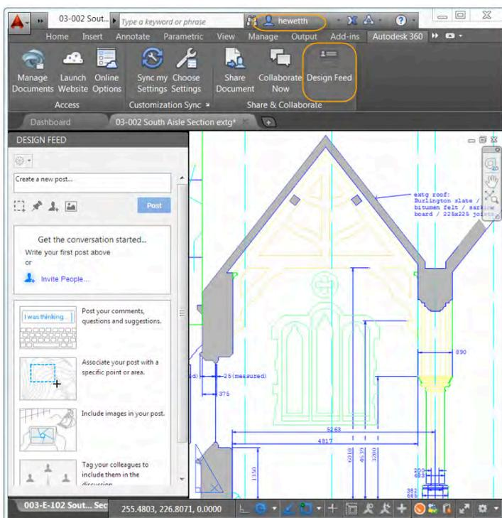
If you associate your comment with a location or area within the drawing, a corresponding bubble is displayed. When you select a comment in Design Feed, AutoCAD zooms to the corresponding part of the drawing. If you select a bubble in the drawing, the corresponding comment is selected in Design Feed. The Settings drop-down menu on the Design Feed palette lets you control the display of the bubbles.
