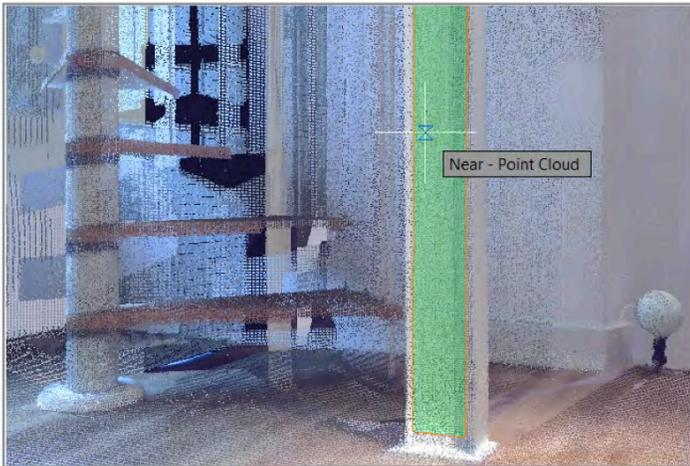
You can use the UCS tool and specify the Object function to align the current UCS to a plane in a point cloud.
