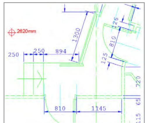
You can control object snap behavior for dimension extension lines with a new option on the Drafting tab of the Options dialog box.
