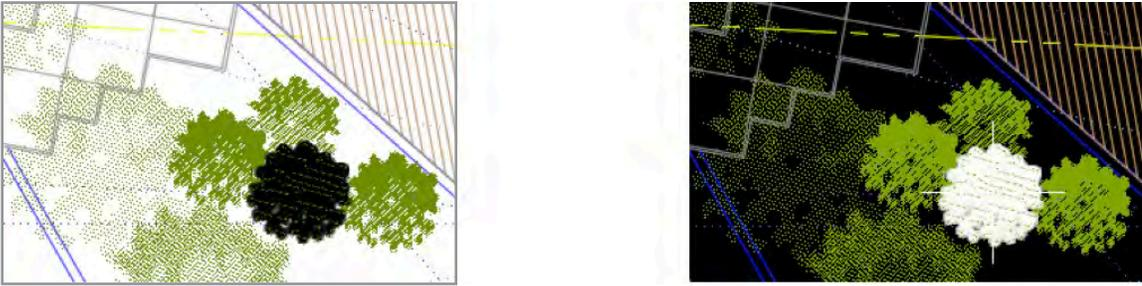
If hardware acceleration is turned on, selecting an object changes its color and it remains thickened to clearly identify it as part of the selection set.
