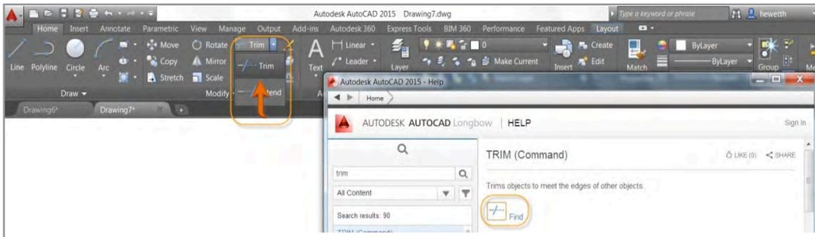
If the tool is not accessible from the current workspace or is located in a hidden tab or panel, a tooltip in the Help window tells you on which Ribbon tab and panel you can find it.
