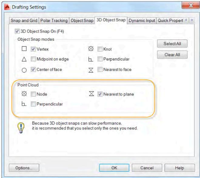
For easier access to point cloud object snaps, customize the status bar to display the 3D Object Snap tool.
