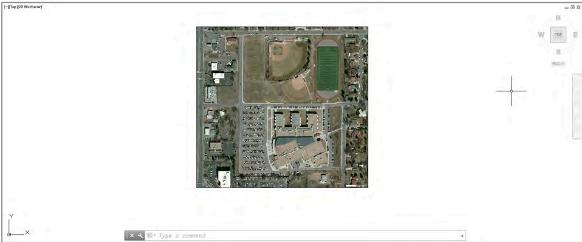
You can select the embedded map image and use grips to move, resize, and even rotate the image boundary. When you change the image boundary, AutoCAD automatically re-queries the online map data and updates the image accordingly. A contextual Map Image Ribbon tab displays additional relevant tools when a map image is selected.
