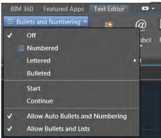
Then when you begin a line with a symbol or with a number or letter followed by one of these characters and a space or tab, AutoCAD automatically creates a bullet or numbered list: ".", ")", ">", "}", ":", or "]". An icon indicates that automatic bullets or numbering has started. You can click on the icon to access relevant controls including an option to remove bullets or numbering. Pressing backspace immediately after pressing the space or tab also removes automatic bullets and numbering.
