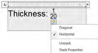
Stack Properties enables you to change additional properties of the current fraction and as well as AutoStack behavior in the enhanced AutoStack Properties dialog box.
