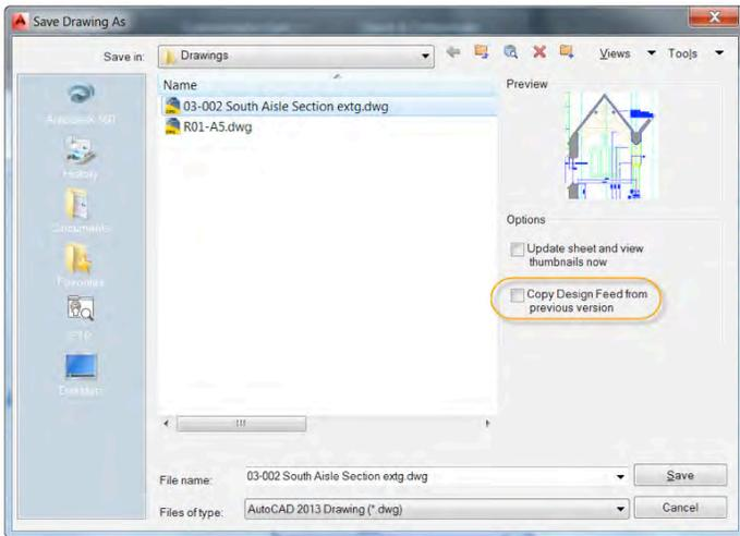
If you create a copy of a drawing using eTransmit, Archive, or DWG Convert, you can specify whether Design Feed data is removed from the drawing using the relevant setup for each of those tools. By default, the option to remove Design Feed is enabled.
