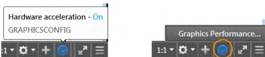
When Hardware Acceleration is turned on, you have access to a variety of controls that can improve the appearance of your display.
