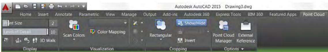
Support for attaching PCG and ISD point cloud file formats has also been removed in AutoCAD 2015. However, if you open a drawing to which those older point cloud files are attached, they will display and you can select them and modify their properties.
