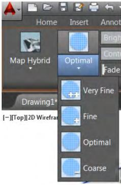
Slider bars on the Map Image Ribbon tab enable you to adjust the brightness, contrast, and fading of the map image so that you can more easily see relevant AutoCAD geometry.
