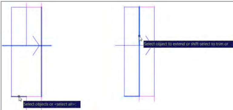
The Lengthen tool also supports command preview. It has been further enhanced in AutoCAD 2015 to default to the last lengthen option (delta, percent, total, dynamic) so you are no longer required to specify an option each time you launch the command.
