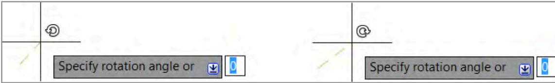
The badge displays a clockwise or counter-clockwise arrow according to the direction specified by the Drawing Units.
