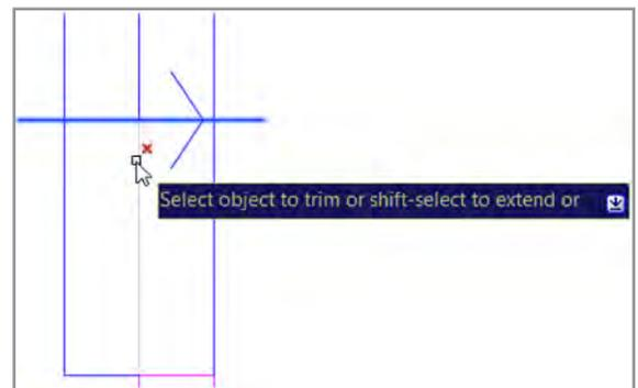
When selecting an object to extend, it is clearly identified and temporarily extended.
