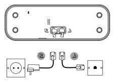
Plug the power adaptor into the socket marked Q: on the underside of the base and plug the other end into the mains power wall socket. Switch on the mains power.
