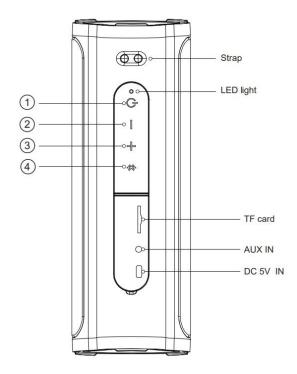
1. Power On/Off/Mode: Long press to power On/Off. Single press to change mode.
