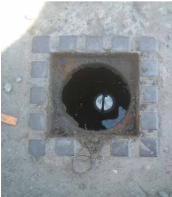
3. Make sure there is a good, clean, magnetic contact to the valve stem or hydrant. For optimum sound and radio transmission deploy the Zonescan vertically. To prevent the Antenna touching the metal lid and reducing transmission, fit a polystyrene block between the lid and Antenna.
