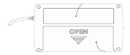
6 Dry cell cover: Cover below which dry cells are put
