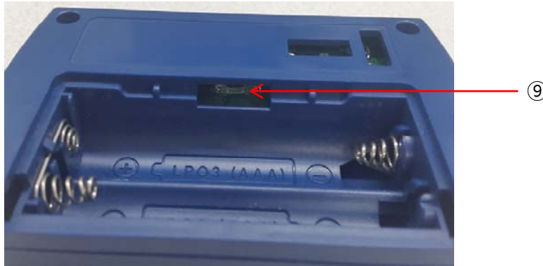
⑨ Hidden button: A hidden button used for Bluetooth pairing
