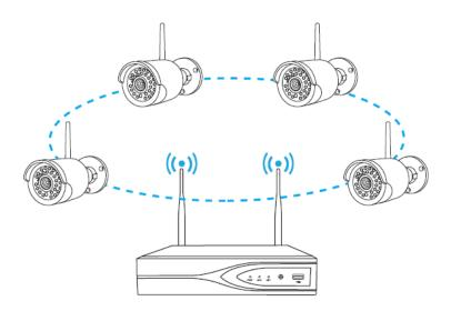
2) If the distance between IPC and NVR is too far, the signal is not strong enough, you can take off the original antenna and substitute antenna extension cord, then put it where WIFI signal is strong.
