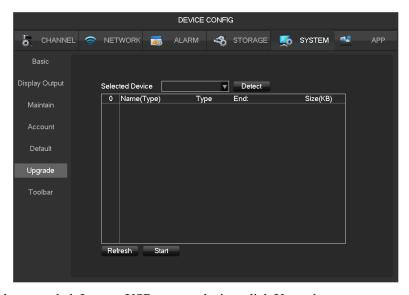
System software can be upgraded: Insert a USB storage device, click Upgrade.
