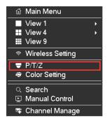
When the NVR is connected with a network PTZ camera, right click the corresponding network channel and select [PTZ] to enter into the PTZ interface.
