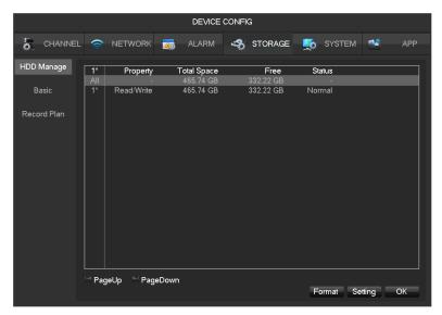
A Hard disk format operation results in the loss of video data.
