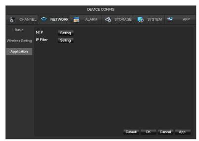
[NTP]Select Enable switch to turn on the NTP protocol support, can be with SNTP communication server to realize automatic calibration function.
