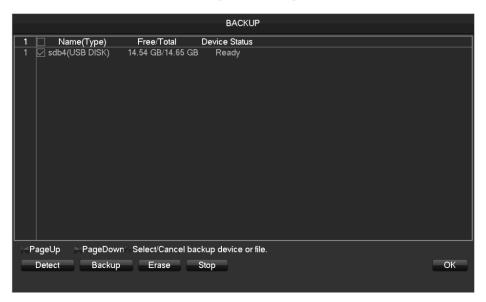
[Detect] Identify external USB device and display the device information.
