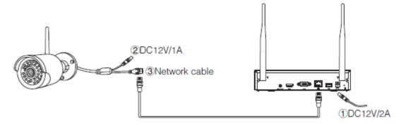
The light of NVR on the wan port interface should be on, if the light is off, then can't match code, please check if the cable or device can work well or not.
