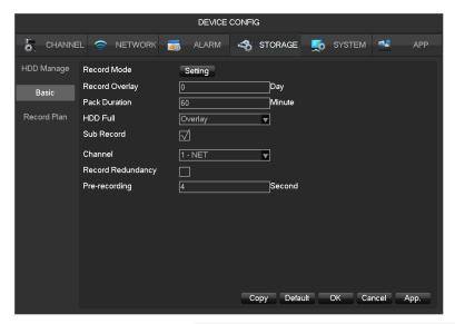
[Record Mode] Support three modes, 'record automatically', 'manually' or 'not record'.
