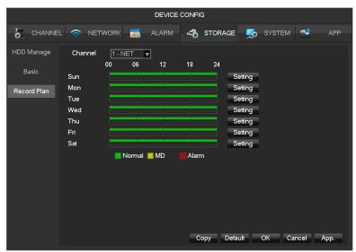
[Channel] Select a channel. Green shows normal recording, Yellow shows motion detection, and Red shows Alarm. Users can set or change setting according to date.
