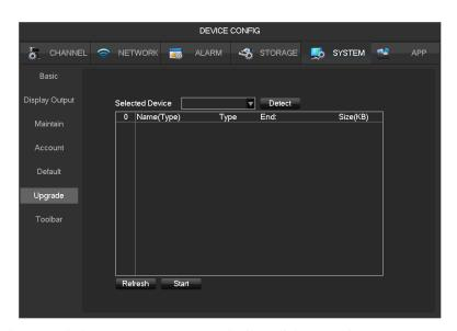
System software can be upgraded: Insert a USB storage device, click Upgrade.
