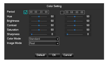
[Period] Two periods can be set according to ambient light during the day and night, device will automatically switch configuration time. Need to select the Enable box.
