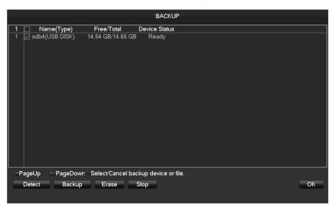
[Detect] Identify external USB device and display the device information.
