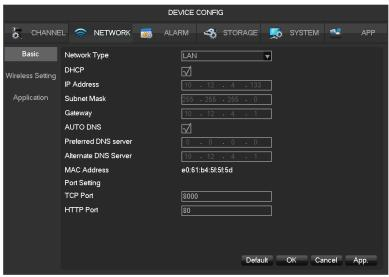
**[DHCP]** Enable the NVR to obtain an IP address automatically. If it is enabled, the NVR will reboot and search for a DHCP server, and then assign a dynamic IP address. The dynamic IP address will be displayed in the menu. Enter a static IP address if there is no DHCP service available. If you are using the advanced feature PPPOE, then the IP/mask/gateway and DHCP are unable to be changed.
