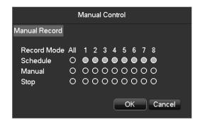
[Manual] The tick boxes in this row have the highest priority and when you have ticked the corresponding channels the NVR will record continuously.
