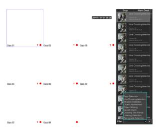
[Filter] Events filter: Face detection, Line Crossing detection, Instrusion detection, Object abandoned, Object missing, Density alarm, Crossing the fence, Loitering detection, Retrograde detection.
