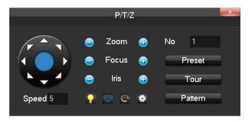
Make sure that the PTZ's protocols support this function. The PTZ will turn to the clicked point and move it to the centre of screen. It also supports zooming into and out of the video image. Drag the mouse in the quick location page to zoom into an area of the footage. The dragged box can zoom in to the image in between 4 to 16 times. Hold the mouse and drag it up to complete zoom of the box. Drag it down to narrow the box.
