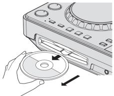
If the [DISCA] button is pressed accidentally, press the [PLAY/PAUSE>/II] button immediately. Disc ejection is canceled and the unit is reset to as it was directly before the [DISCA] button was pressed. (No sound is output during the resetting process.)
