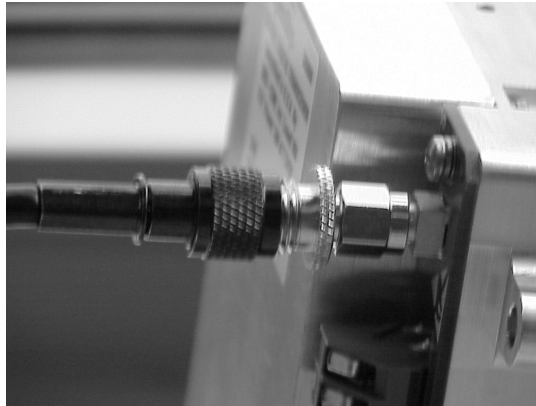
Figure 5-2: Antenna Wire Connector Installed
