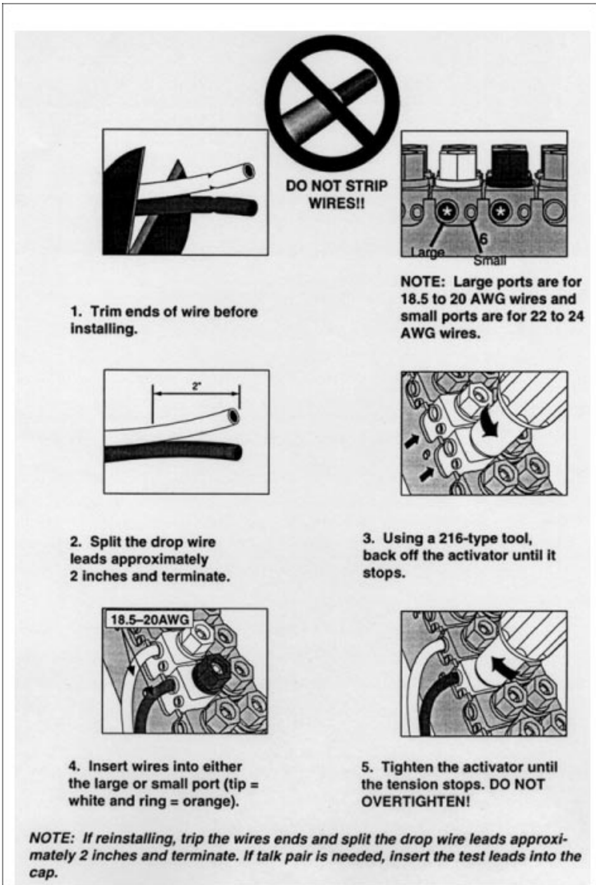
Figure 4-16. Terminating Wires in TI Surge Protector
