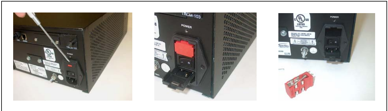
Figure 4-3: CS-7200 Fuse Replacement (Rear Panel Views)
