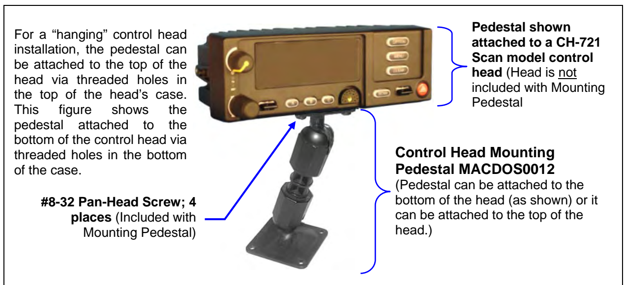
Figure 9-5: Optional Control Head Mounting Pedestal (Part Number MACDOS0012)
