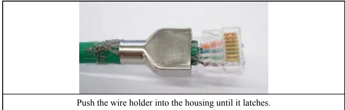
Figure D-15: Cable Positioning, Latch Wire Holder in Housing
