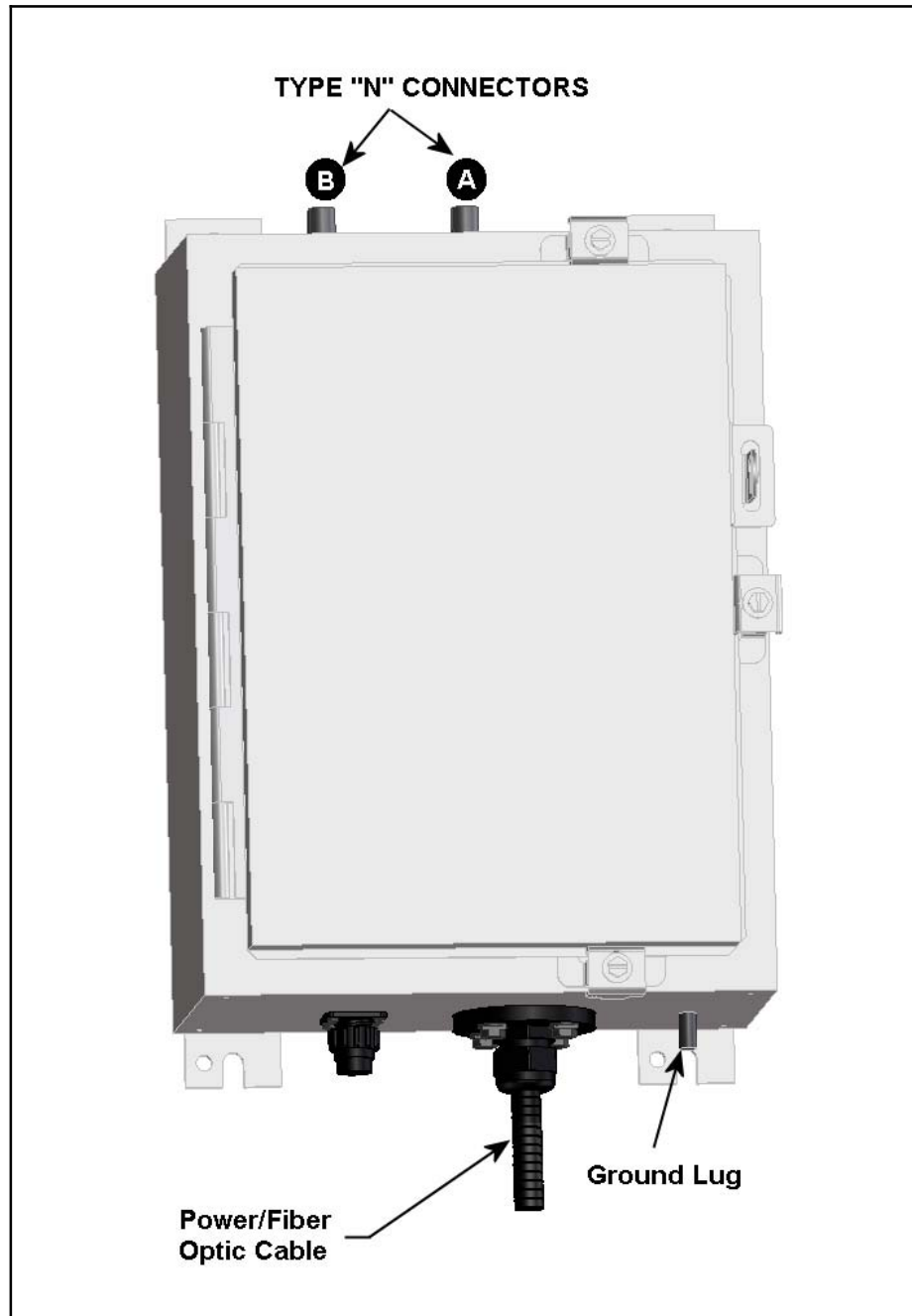
Figure 6-1: ISM Tower Top Radio Enclosure
