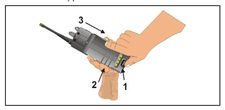
Figure 22: Removing the Battery Pack
