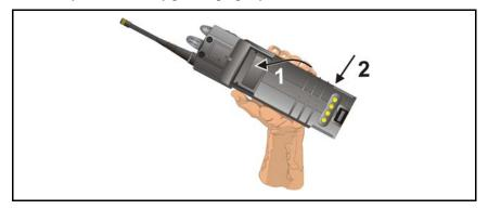
Figure 23: Attaching the Battery Pack
