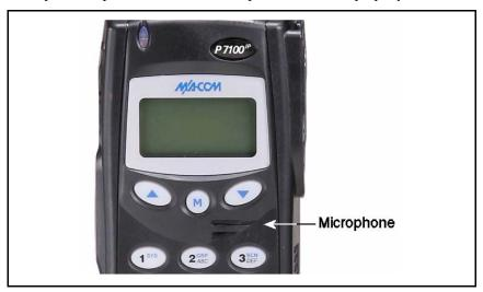
Figure 21: Radio Microphone
