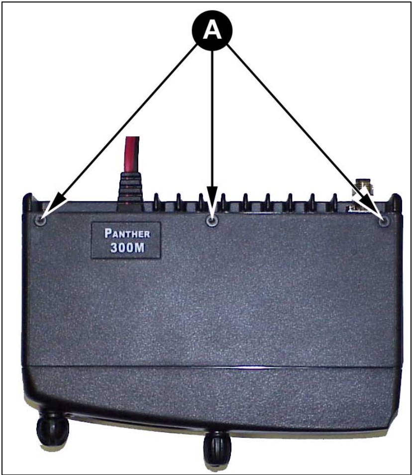
Figure 2 – Removing Top Cover
