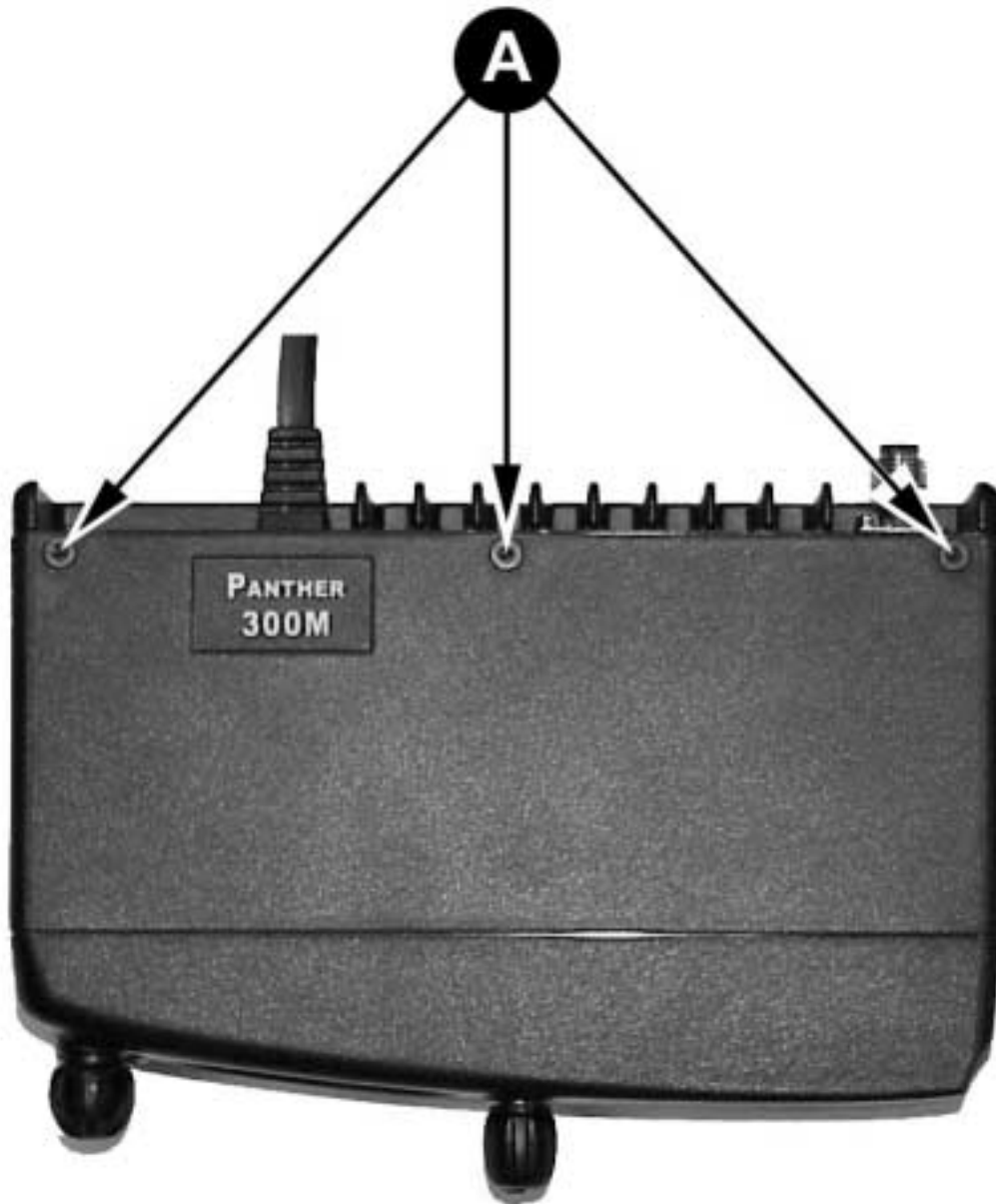
Figure 2 – Removing Top Cover
