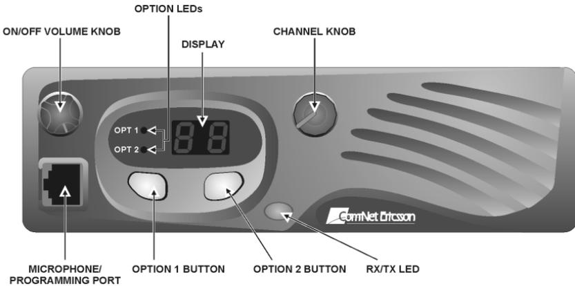
**Figure 1 – PANTHER 300M mobile radio Front View**
