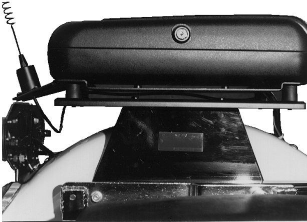
Figure 6 – Case Mounting Bracket and Case Assembly
