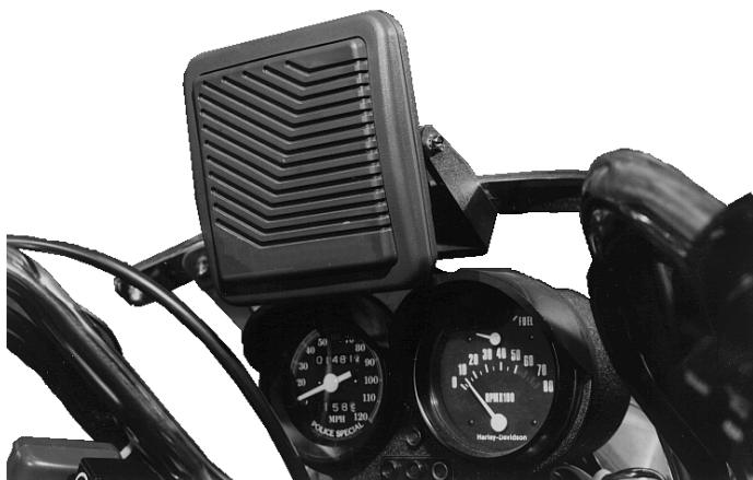
Figure 10 - Typical Speaker Mounting
