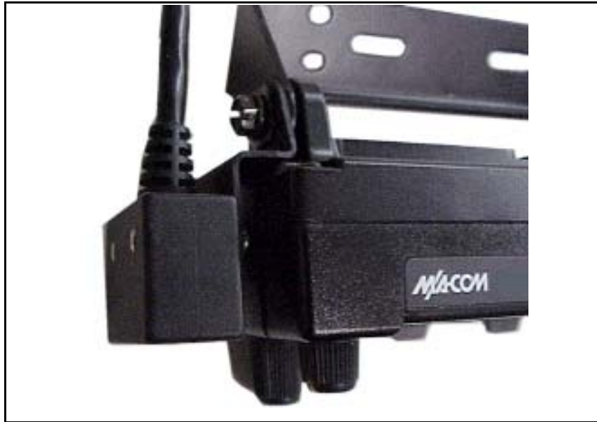
Figure 15 – Pigtail Bracket Installed on Control Unit
